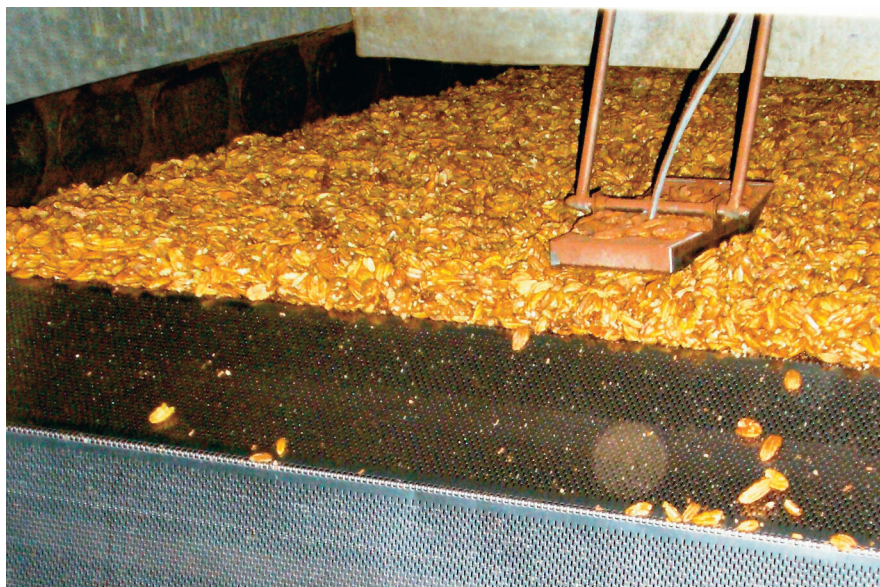
The flat-plate moisture sensor's hinged mounting device enables the sensor to ride over the kernels' tops, regardless of the material-bed depth.
