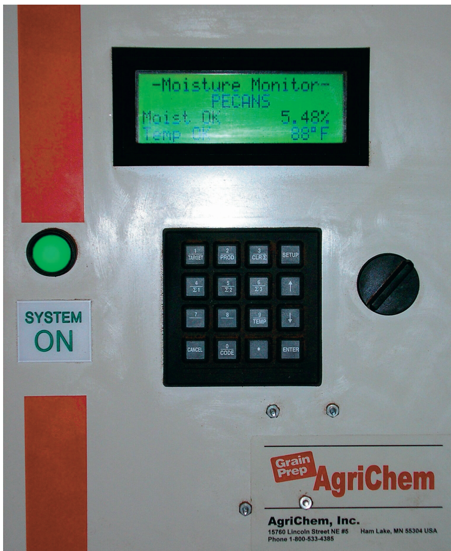
The sensor monitor continuously displays the kernels' moisture-content and current-status readings as they discharge from the dryer.
