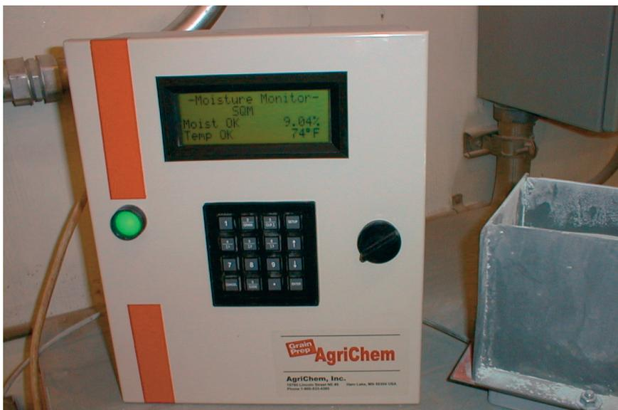
***The monitor receives a signal from the sensor and converts it to moisture content and temperature readings that are displayed on an LCD screen.***
