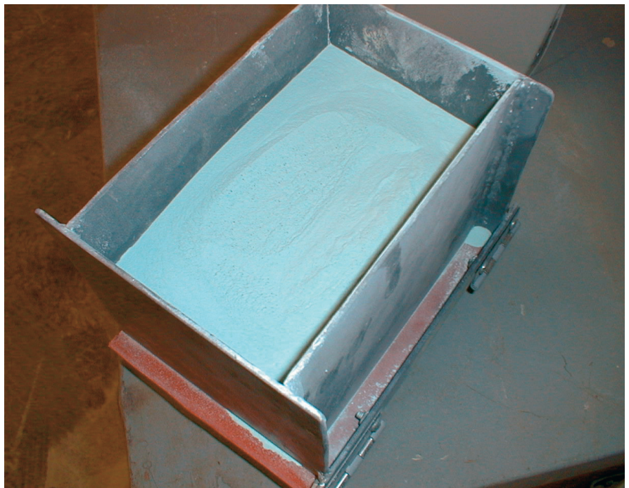
For this application, the moisture sensor is mounted in the base of a box, allowing the company to use it as a benchtop unit for material testing.
