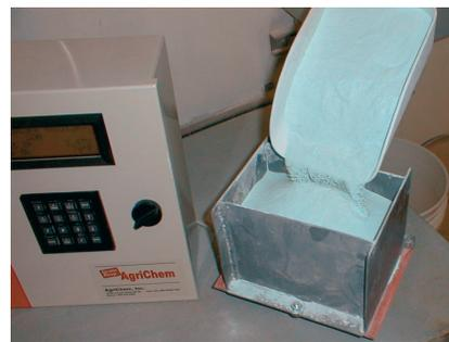
**The sensor and monitor are located on a table next to the bagging machine, allowing an operator to quickly determine a product’s moisture content.**
